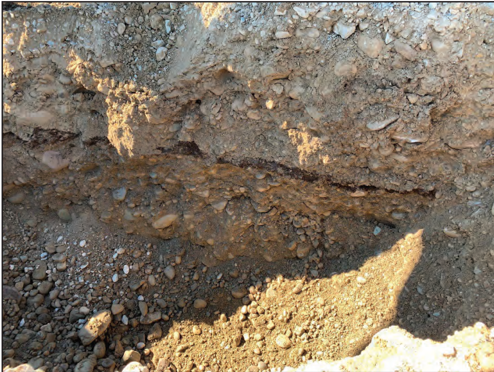
Photo 4: Test pit on Lot 73. Existing granular fill is exposed over thin dark topsoil and medium brown sandy gravel (March 16, 2021).
